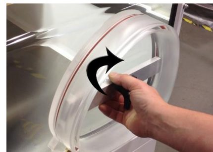
Figure 21: Securing the Arm Port Doors
