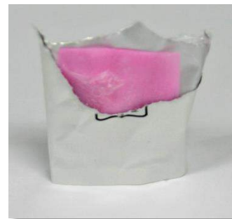
Figure 23: Pink indicating the presence of oxygen in an office environment
