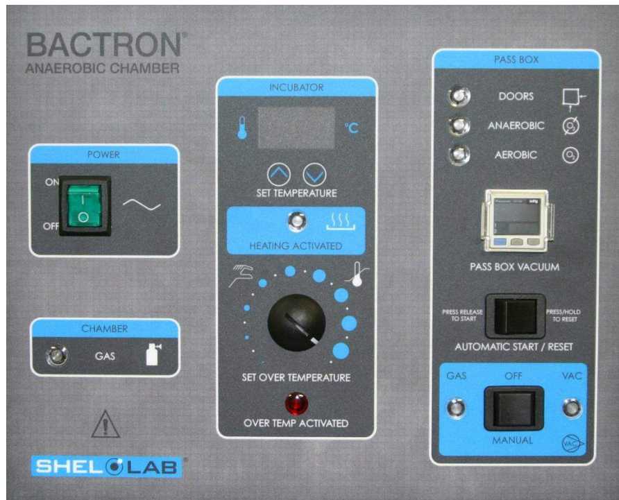
Figure3: Main Control Panel
