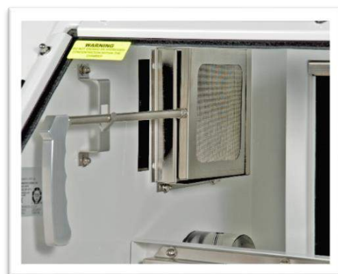
Figure 22: Catalyst Cartridge Installed
